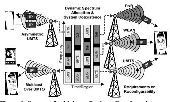
Figure 1: Support for high quality broadband services in a reconfigurable multi-radio environment
